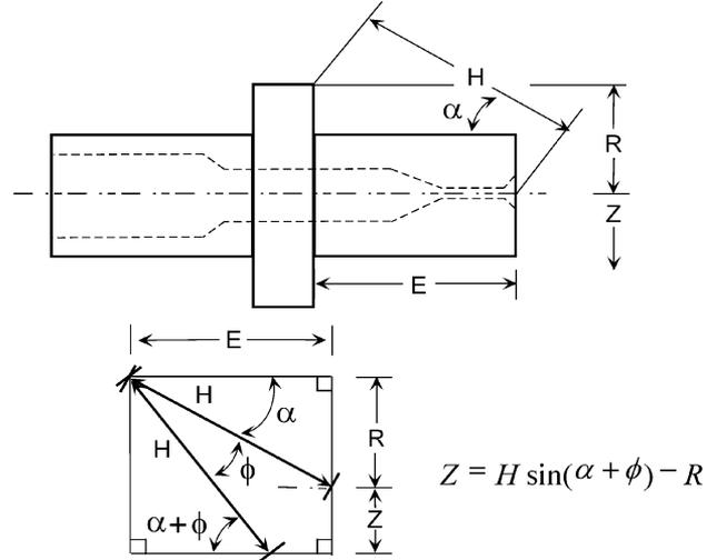
Fig. 10. Geometry of fiber tip motion due to angular rotation of ferrule about the weld.
