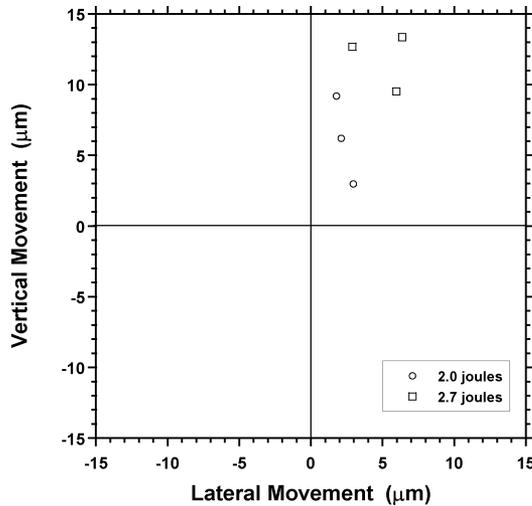
Fig. 2. Effect of laser pulse energy on ECS measured post weld shift for butt-welded alloy ferrules. No restraint applied, weld position #3.
