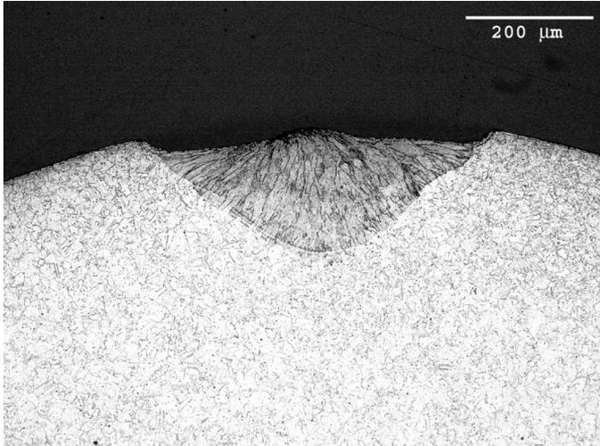
Fig. 9. Optical micrograph of typical laser spot weld between Kovar ferrule and sleeve. 1.2 J, 2 ms.
