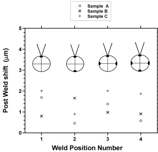
Fig. 8. Effect of weld position and location of prior spot welds on resultant post weld shift magnitude. 1.7 J, 2.0 ms, 1.0 kN load.
