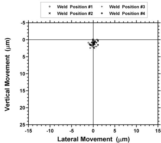
Fig. 5. Post weld shift of restrained Kovar ferrules as measured with CCD camera. 1.7 J, 2.0 ms. Initial fiber tip location at (0,0).
