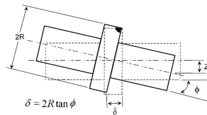
Fig. 6. Rotational movement of optical ferrule due to transverse shrinkage of weld. Movement is exaggerated for clarity.
