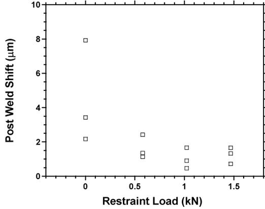
Fig. 7. Resultant post weld shift magnitude of Kovar ferrules as measured with CCD camera. Weld Position #2, 1.7 J, 2.0 ms.
