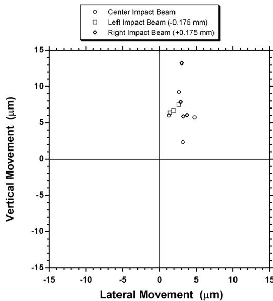
Fig. 3. Effect of beam position on ECS measured post weld shift for butt-welded alloy ferrules. No restraint applied, weld position #2.
