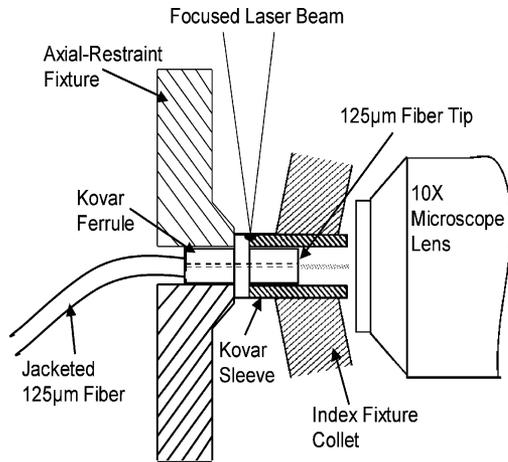
Fig. 1. Experimental setup for spot welding, restraint application, part rotation, and camera imaging of post weld shift.
