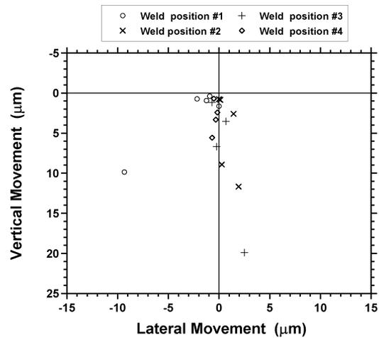
Fig. 4. Post weld shift of unrestrained Kovar ferrules as measured with CCD camera. 1.2 J, 2.0 ms. Initial fiber tip position at (0,0).
